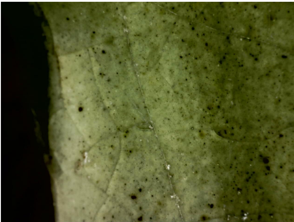
Impurities into the core material as into the glaze. Also typical cracks into the glaze (magn. x100)
